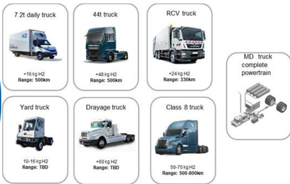
FIGURE 1 HYDROGEN STORAGE AND VEHICLE DRIVING RANGE IN VARIOUS COMMERCIAL TRUCK PLATFORMS. REF.: S. KNIGHTS, “ZERO EMISSION FUEL CELL TRUCKS,” IEA TCP-AFC TASK 34 MEETING, DECEMBER 12, 2022.
