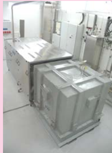
Figure 10. 10 kW SOFC system at VTT, Finland.
