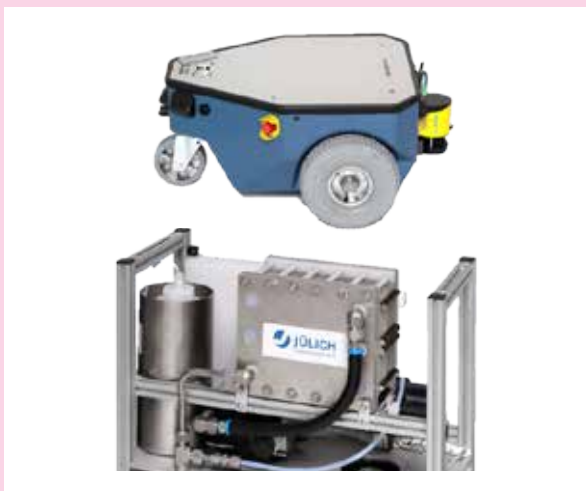
Figure 29 Service robot (top) and DMFC system that is integrated into the robot at Forschungszentrum Jülich, Germany (Source: Forschungszentrum Jülich) (bottom).
