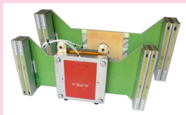
Figure 28: Picture of the developed sensor board, TU Graz (Source S++).
