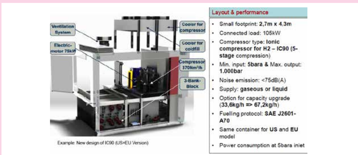
Figure 22: Hydrogen fuelling station for serial production: the Linde Group IC90 Ionic Compressor
