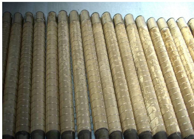
Figure 20. 36-tube bundle for a 300 W portable power unit [source: www.Msri.com]
