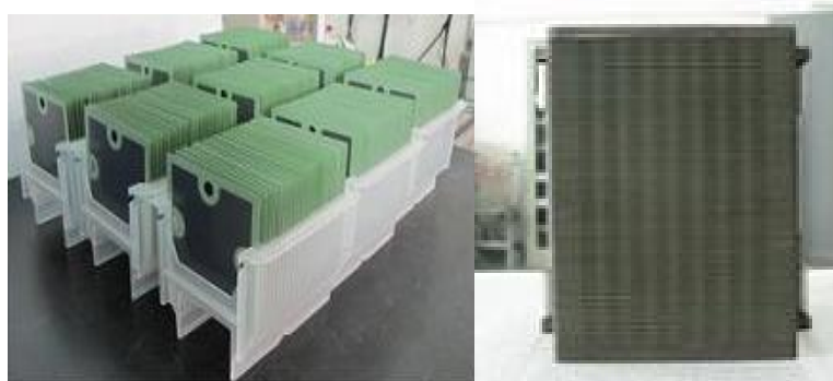
Figure 59. SOFC electrolyte supported cells and the SOFCMAN-ASC 60 Cell stack 601 with 10 cm*10 cm cells, maximum output power: 1600–2000W at 750°C, operation power :1400–1600W at 750°C, 0.70–0.75V
