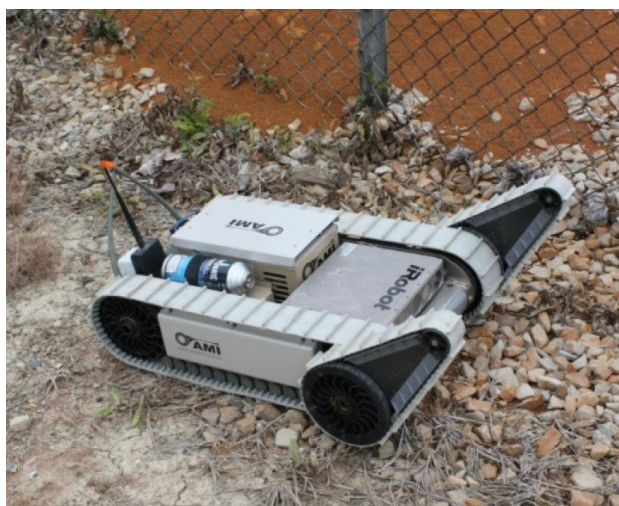
Figure 5. The iRobot PackBot UGV AM is a reconnaissance unmanned system, capable of 12 hours autonomy covering about 40 miles of terrain. This System is hybridized with a standard battery for 2.5 hours (8 miles) extra autonomy [source: Ultra-AMI, Proceeding of Fuel Cell Seminar and Exposition 2011]
