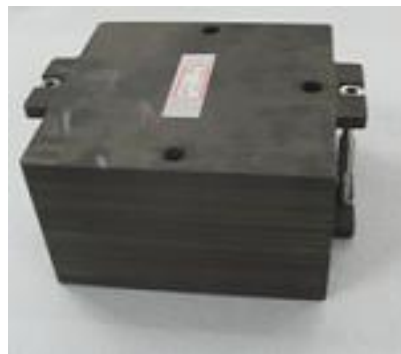
Figure 60. SOFCMAN-ASC 30-cell Stack-2kW in this product the cell area is enlarged from 10cmX10cm to 14cmX14cm, SOFCMAN 30-cell stack (14cmX14cmX8cm) with double area showed a peak power of 2.6kW and current of 128A at 750°C. Under a self-sustained condition, the stack power reached 2.2kW, at a current of 90A, average cell voltage of 0.8V, fuel utilization of 68%, and electric efficiency of 44%. The volumetric power density is over 1.4kW/L.
