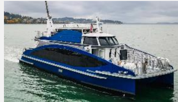
Sea Change, 2023. 3 x 120 kW PEM fuel cell 242 kg, 250 bar.
