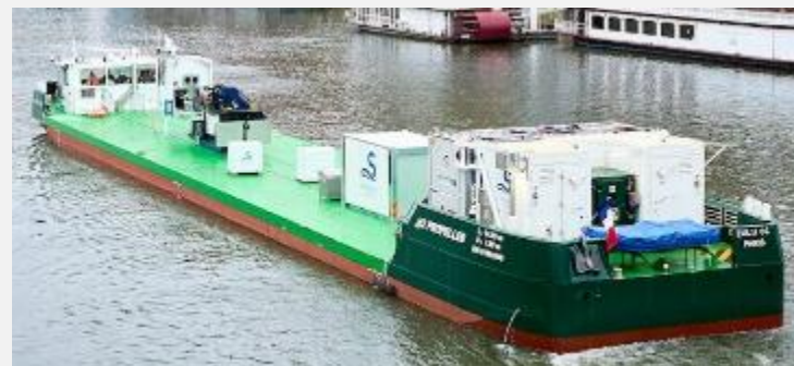
Zulu 06, PEM FC 2 x 200 kW., 280 kg Hydrogen, 300 bar, 14 m 3
