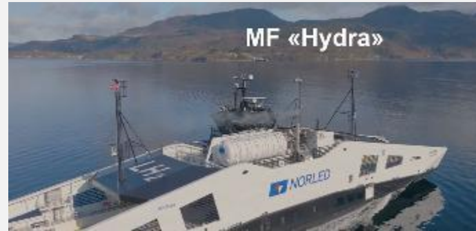
MF Hydra, Norled. 2021 Liquid Hydrogen (4T, 56 m 3 ). 2x200 kW PEM fuel cell.
