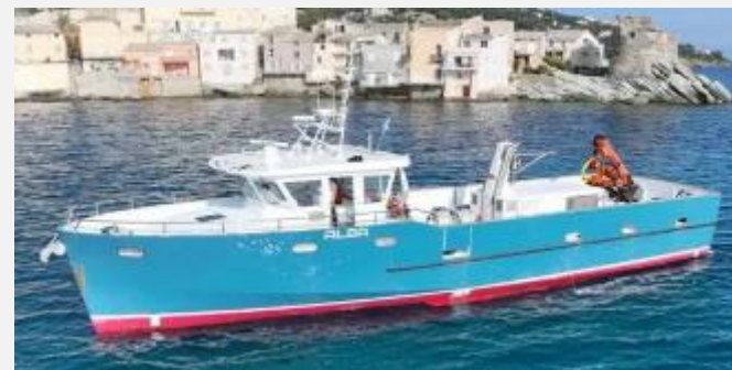
Alba, 2 x 70 kW PEM fuel cell, 2024 350 bar, 75 kg.
