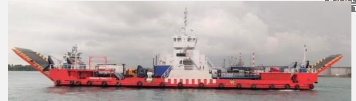
Penguin, Demonstrator. VINSSSEN 60kW FC. Compressed H 2
