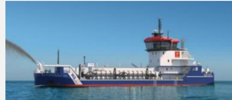
Dredger “Hydromer”, 2024 200 kW PEM fuel cell 500 bar, 2 T.
