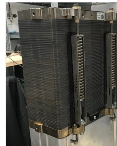
65 cell stationary stack with Ion Pair (165 cm 2 active MEAs) Similar lifetime
