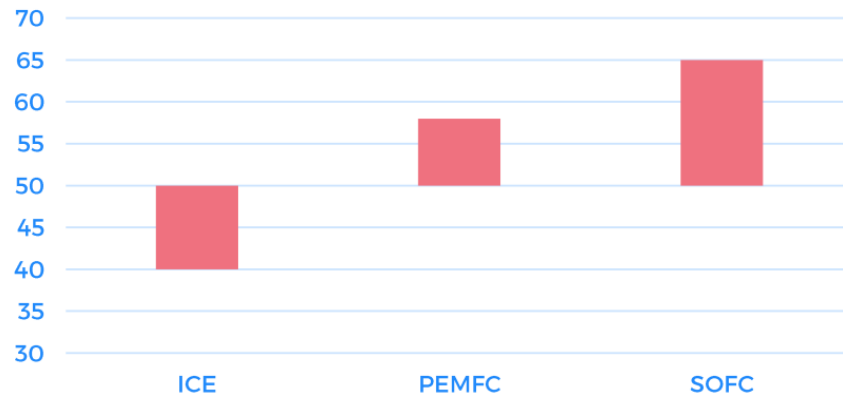
Figure 19. Electrical efficiency comparison of an internal combustion engine with PEMFCs and SOFCs
